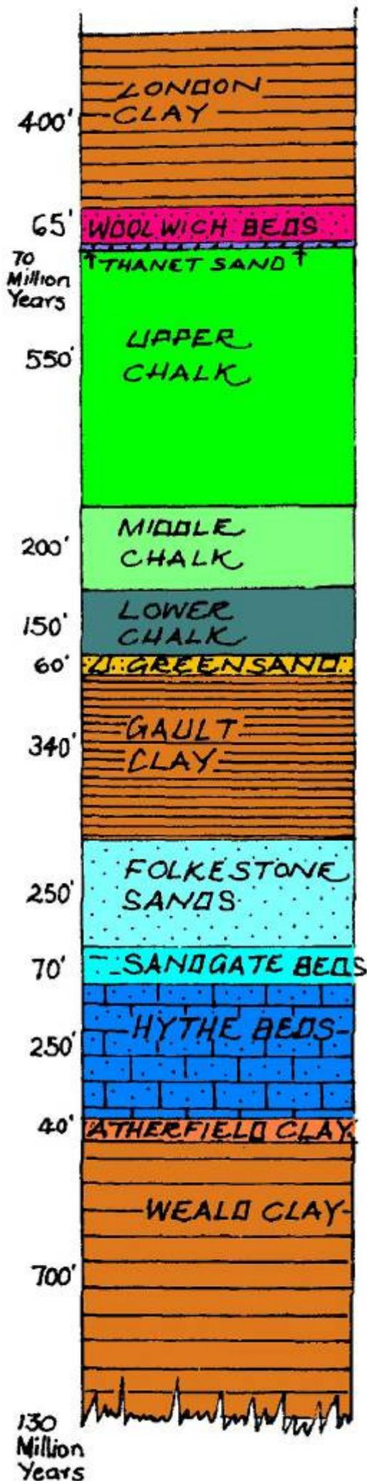
cross-section of the local landscape running from north to south. It shows how the chalk fits into the overall geology of the area. The picture to the left shows the thickness and age of the different rock types.
